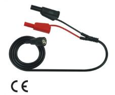
Feture:Insulated BNC Male to 2\*4mm stackable safety plugs,connected with the flexible RG58/50  $\Omega$  wire.L:1.2M
